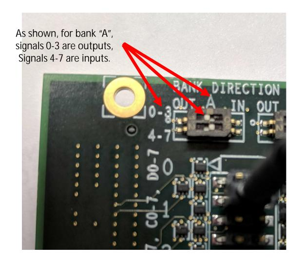
The DIP switches control the signal direction for a bank of 4 pins. Move the slide towards the word "OUT" to make an output bank. Move the slide towards the word "IN" to make an input bank.
