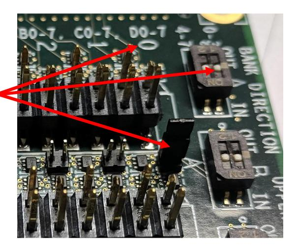
The 2-pin headers are used to add a 50 ohm input termination to a channel. Insert a jumper to connect the 50 ohm resistor. Remove a jumper to leave the channel with only a 1k pull-down resistor to ground.
