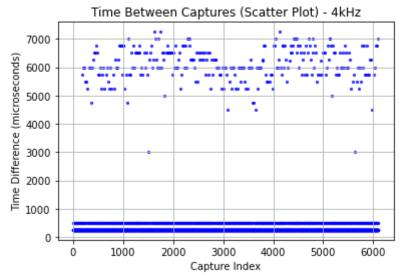
Average: 557.02 microseconds Standard Deviation: 1245.64 microseconds Average (Hz): 1795.26 Hz
