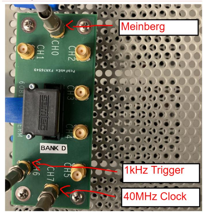
Copies of D0-D3 triggers are sent out of D0-D3, while D4-D7 should be configured to be input signals. The trigger input should go to D6 (It does not have to be 1kHz). A 40MHz clock should go in D7.
