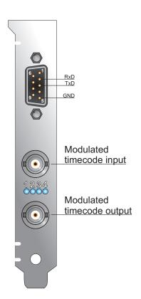
The bracket of the board includes the BNC connector for the amplitude modulated time codes, four LEDs and a 9 pin D-Sub-plug.
