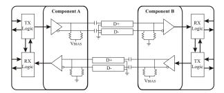
This design leads to a full duplex connection clocked with 2.5 GHz capable of transfering a data volume of 250 MB/s per lane in each direction. Higher bandwith is implemented by using multiple lanes silmutaneously. A PCI Express x16 slot for example uses sixteen lanes providing a data volume of 4 GB/s. For comparison: when using conventional PCI the maximum data transfer rate is 133 MB/s, PCI-X allows 1 GB/s but only in one direction respectively.
